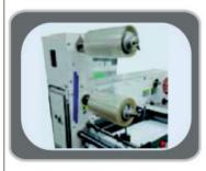
**Optional rewinder for lamination film** Optional rewinder to support lamination film (Backliner).
